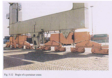
Fig. 5.12 Bogie of a portainer crane.
